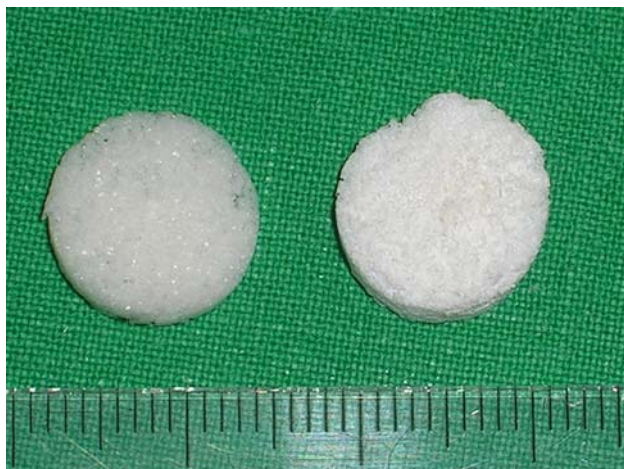
Fig. 1 Images of poly-lactic-glycolic acid (PLGA) scaffold ( left ) and poly-lactic-glycolic acid-hydroxyapatite (PLGA-HAP) composite scaffold ( right ). Scaffolds are cylindrical, 12 mm in diameter and 2 mm in height
